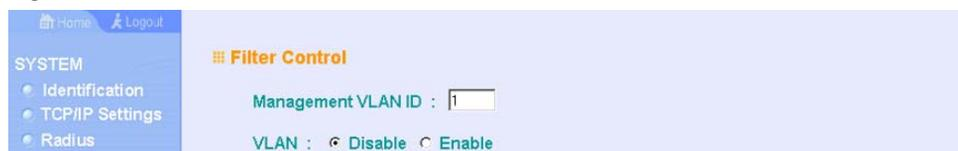
**VLAN** – Enables or disables VLAN tagging support on the access point.
